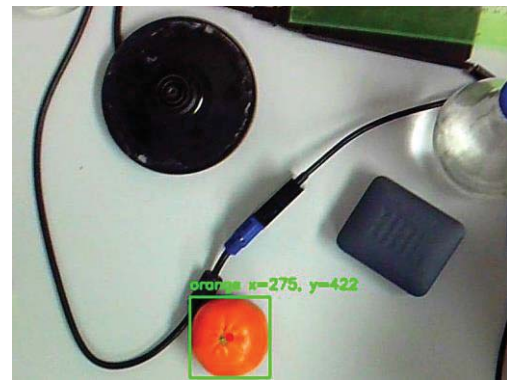
Fig. 3. Overhead camera frame with OpenCV/YOLO overlay showing the detected object (bounding box and center (x,y))
